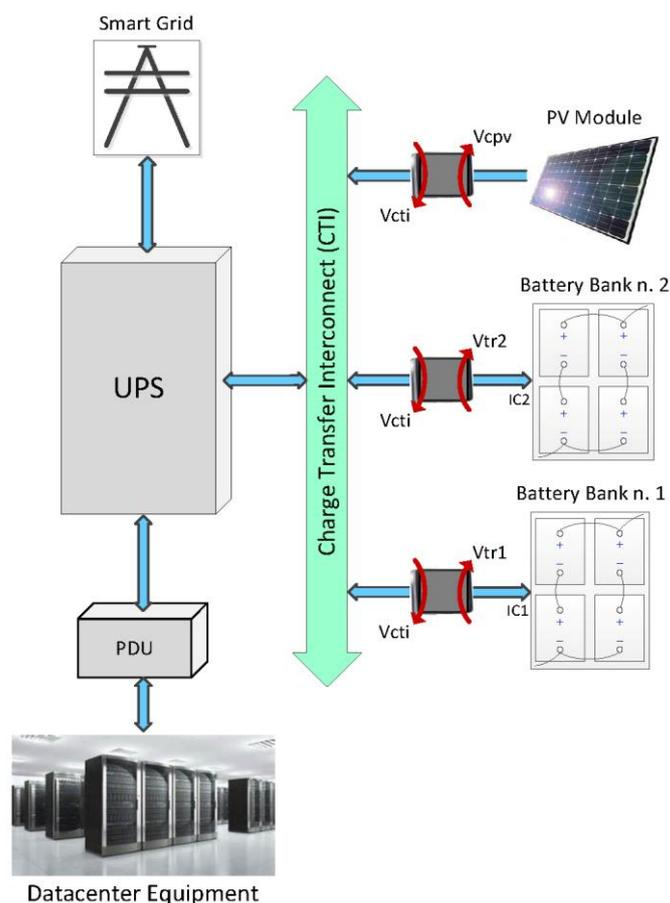
**Figure 1.1 – Modelled green data centre structure (including only IT Infrastructure, but not the data centre building modelling and controller, described in Deliverable 3.7 – “Smart Energy Management System”)**
