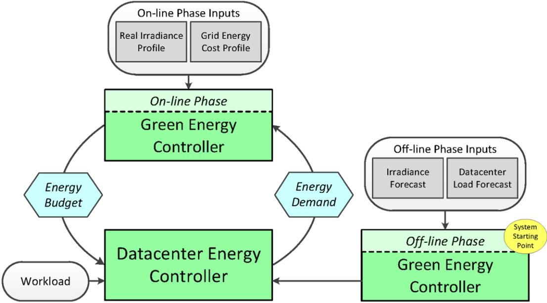
**Figure 1.2 – Diagram of the Electricity Consumption Forecasting Tool, showing the Green and IT Infrastructure Energy Controllers (i.e., used as parts of the data centre building modelling and controller, which will be described in Deliverable 3.7 – “Smart Energy Management System”**
