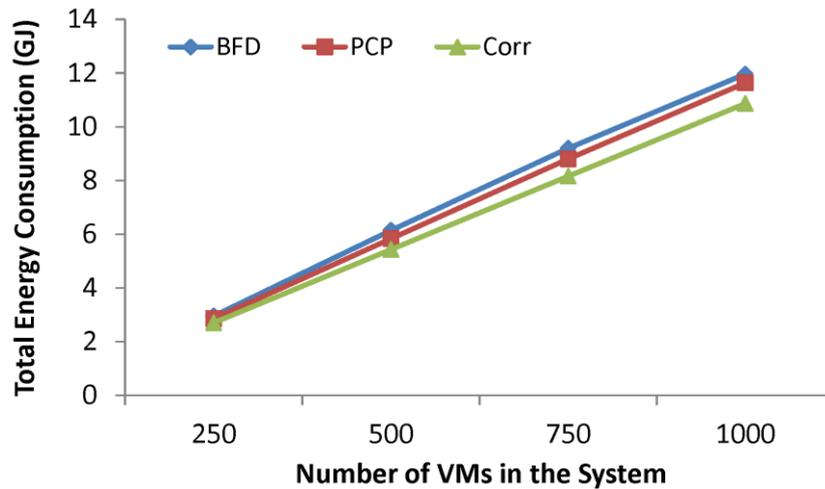
Fig. 4.2 – Total energy consumption of data centre under different number of VMs for a horizon of 14 days
