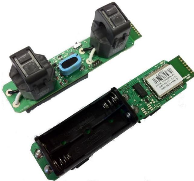
The current measurement range is 0 – 32A, with a resolution of 40 mA.
