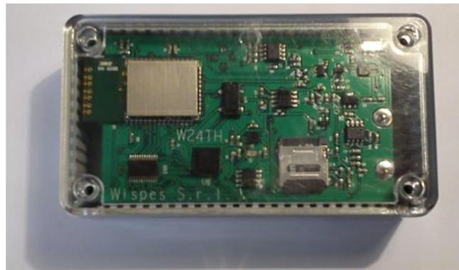
The W24TH node is provided with a series of on-board sensors:
