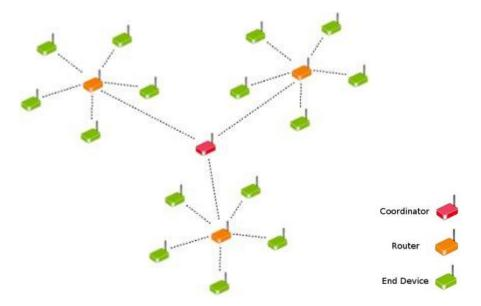
The main network protocol used in our WSN is based on the IEEE 802.15.4. Within the WSN there are mainly three types of wireless nodes (see the above figure):
