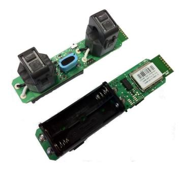
The current measurement range is 0 - 32A, with a resolution of 40 mA.
