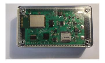
The W24TH node is provided with a series of on-board sensors:
