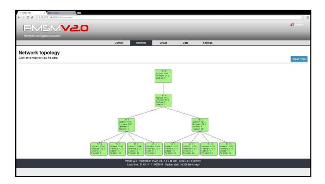
This page shows also the main nodes information, like the node ID, the node network address, the node firmware version, and its transmission timeslot. The color of the node is associated to its state, as well as its battery state.
