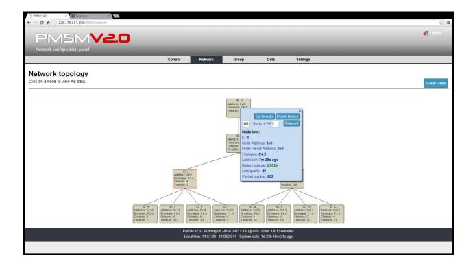
This feature enables a very easy and intuitive network creation with just very few user clicks. The same functionality can be used for modifying the network topology, like removing or moving nodes or entire network branches.
